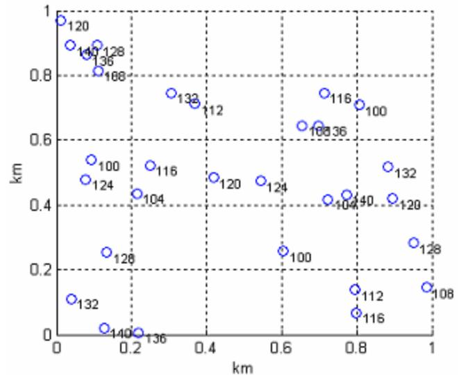
Figure 1: Steady-state Channels Selected for a Random Distribution of Access Nodes with Random Initial Channels in the 5.47-5.725 GHz Band.
